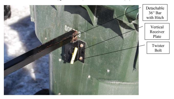
When you have completed pulling container to location, loosen the Twister bolt and **REMOVE** Detachable 36" Bar with Hitch.
